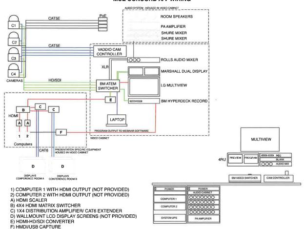
Diagram of wiring types and cable paths. All wiring to be concealed inside walls and equipment racks. Desktop equipment for video control unit will hidden under a hinged counter, only visible when in use. Finish materials pending upon release of design guidelines.
